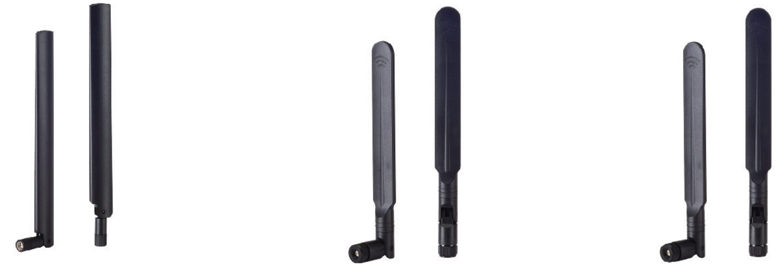
EM-674 specification Frequency: 824-960/1710-2170/ 2600-2700 MHz L=201mm Connector: SMA M EM-502 specification Frequency: 824-960/ 1710-2170-2700 MHz L=233mm Connector: SMA M EM-500 specification Frequency: 824-960/ 1710-2170-2700 MHz L=173mm Connector: SMA M
